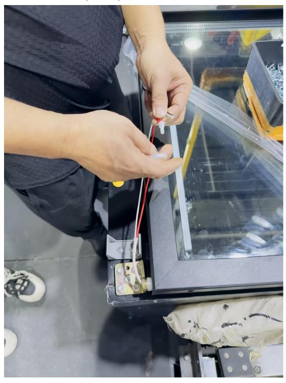
8. complete re-connect the wires and connector
