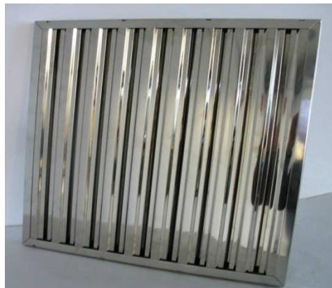
Baffle filters are normally used as a filtering medium in commercial kitchen hoods. The fat particles, heavier than the air, bump against the filter profiles and deposit on those internal surfaces.
