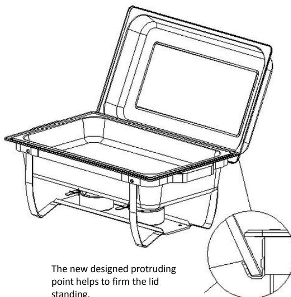
The new designed protruding point helps to firm the lid standing.
