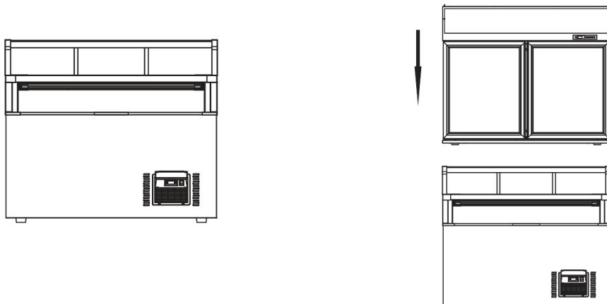
3. After aligning the hole location at the bottom cabinet and the top cabinet as pictures shows, screw up the adjustable foot (M8x50) to the hole position indicated, fix the top cabinet on the platform steadily. The operation requests helper top cabinet.
