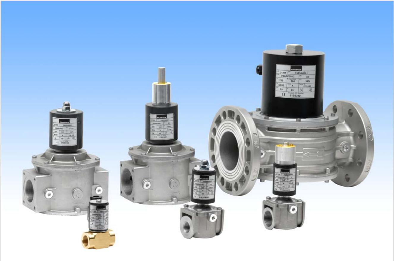
Gas safety solenoid shut-off valve series VSB and VSA, approved according to the Norm EN 161 with **CE** product identification and manufactured according to Atex rule 94/9/CE - Zone 2 and 22 (II 3G – II 3D), are suitable for the automatic control of gases belonging to the first, second and third family. On request there are versions for biogas and air. These valves, normally closed for continuous and cyclic operation, open by powering the coil and close quickly when there is no tension.
