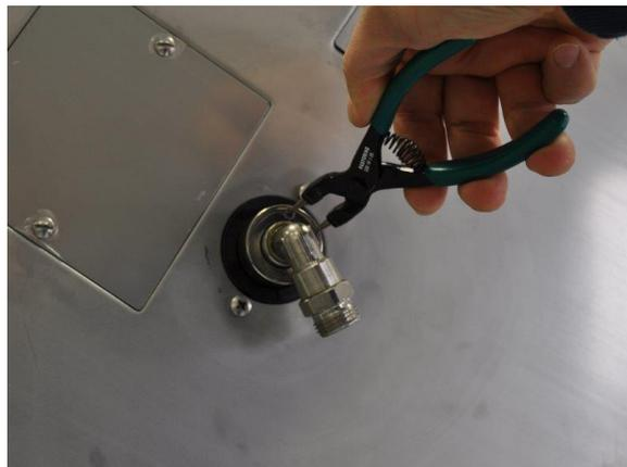
3) Connect the inlet flexible hose to the inlet unit M $\frac{1}{2}$ "G of the MAXIReel.
