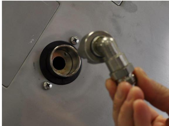
13.4.2. Assembling the inlet unit (elbow connector)
