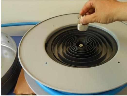
4) Remove the retraction spring.
