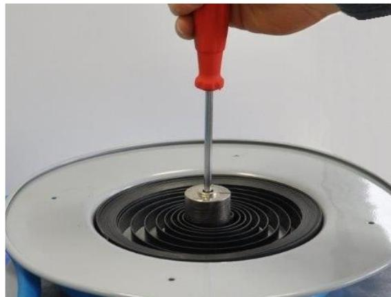
4) Assemble the spring cover and tighten the four M4 screws.
