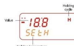
In this exemplum the set point of the holding cycle is modified.
