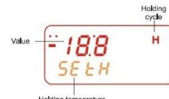
In this exemplum the set point of the holding cycle is modified.
