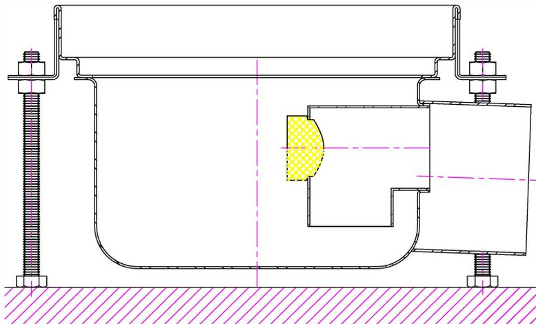
\* THE DRAINAGE CHANNEL IS CONNECTED TO THE PVC PIPE. PLEASE MAKE SURE TO HAVE THE REQUIRED SLOPE AND THE ANGLE OF FLOW.
