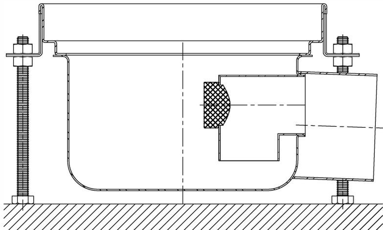
\* THE FLOOR DRAIN IS CONNECTED TO THE PVC PIPE. PLEASE MAKE SURE TO HAVE THE REQUIRED SLOPE AND THE ANGLE OF FLOW.
