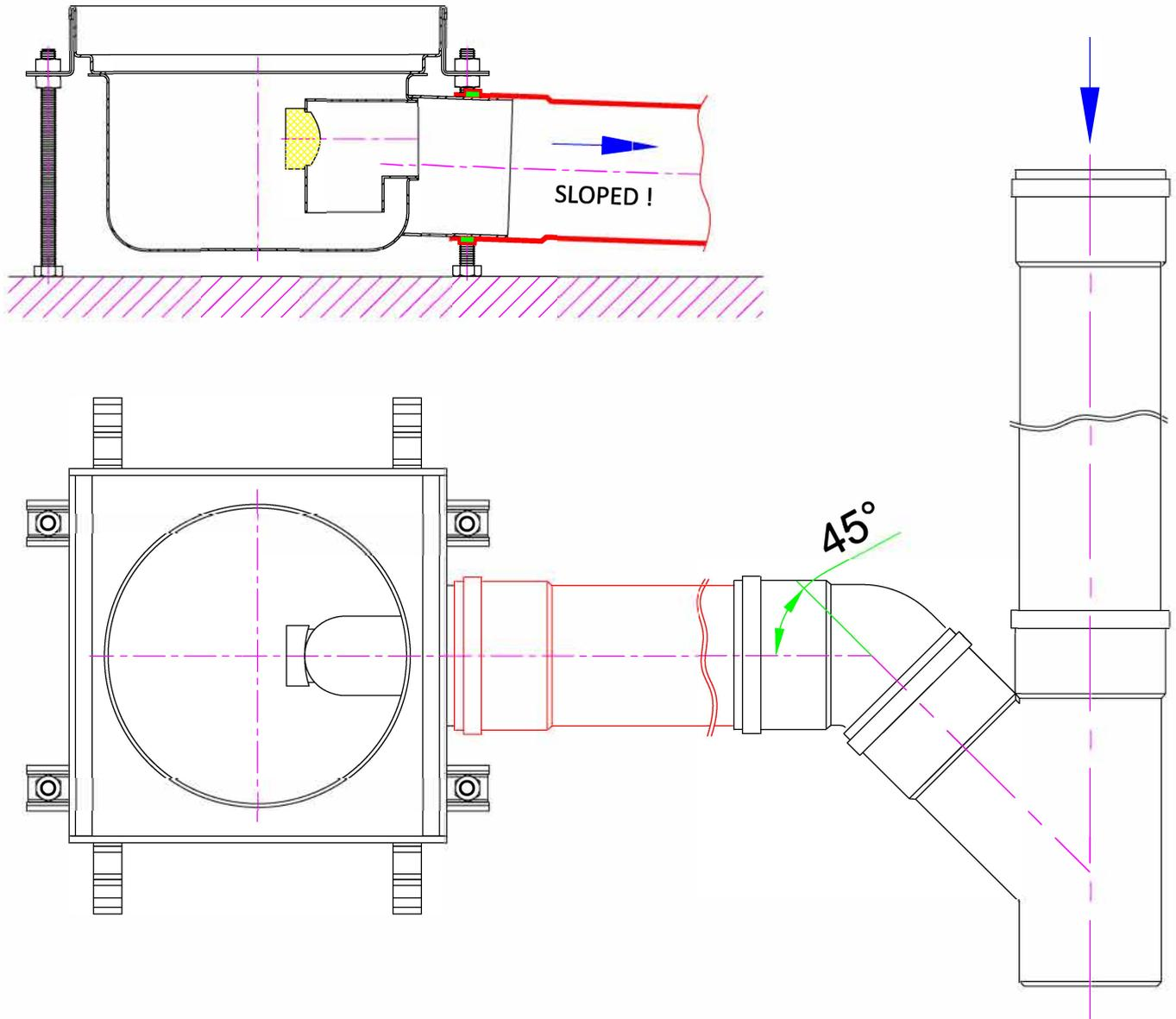
\* APPROXIMATELY 30-40 MM OF CONCRETE IS POURED AT THE BOTTOM OF EACH FOOT AND LEFT TO CURE. MAKE SURE THAT THE FLOOR DRAIN IS KEPT UNTOUCHED TILL THE CONCRETE IS PROPERLY CURED.
