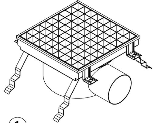
**IT IS RECOMMENDED TO KEEP THE GRATE AND THE FILTER ELEMENT AWAY FROM THE INSTALLATION AREA UNTILL FINISHING THE FLOOR COVERING.**
