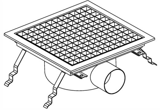
**IT IS RECOMMENDED TO KEEP THE GRATE AND THE FILTER ELEMENT AWAY FROM THE INSTALLATION AREA UNTILL FINISHING THE FLOOR COVERING.**
