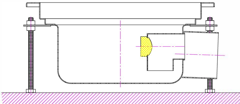
**\* THE FLOOR DRAIN IS CONNECTED TO THE PVC PIPE. PLEASE MAKE SURE TO HAVE THE REQUIRED SLOPE AND THE ANGLE OF FLOW.**
