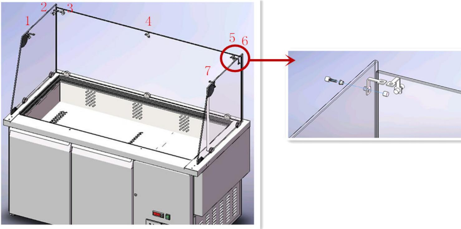
4. Install the top glass by L shape bracket.
