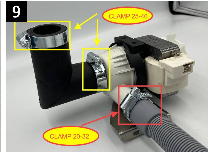
ATTACH THE PUMP HOSE AND THE DRAINING HOSE ON THE DRAINING PUMP
