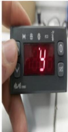
After entering the «LOC» parameter, adjust the «eye» command and press the set button again and return to the main screen by pressing the «Stand-By» button indicated by the arrow in the picture.
