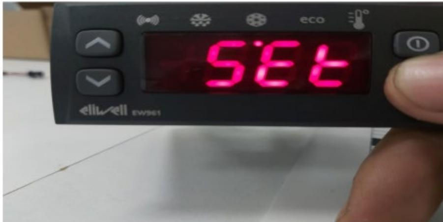
Press and hold the «set» button on the control panel for 5 seconds
