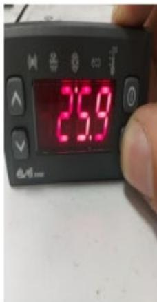
Press the «set» button once from the main screen, after the set text is displayed on the screen, press the «set» button once again to switch to the set change screen.
