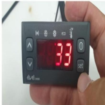
Go to PA1 parameter and press «set» key once Type the password '33' with the up arrow key and press the set key again.
